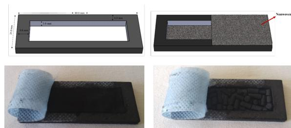
**Figure 2.** A schematic diagram and pictures of ACC and GAC filter holder
